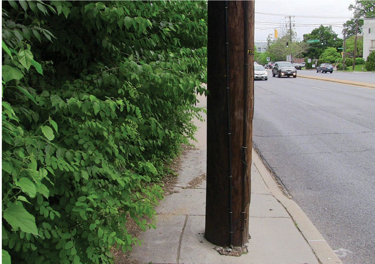
Figure 35: Example Of A Utility Pole Blocking A Sidewalk. Source: American Planning Association.
